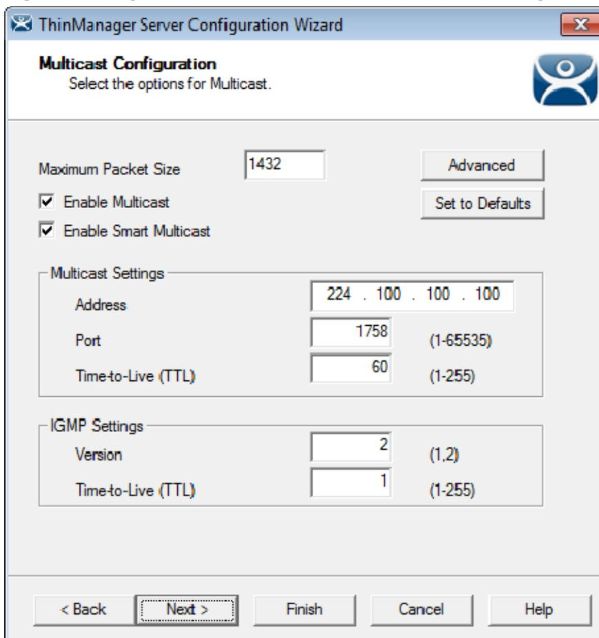
The screenshot shows the 'ThinManager Server Configuration Wizard' window, specifically the 'Multicast Configuration' step. The window title is 'ThinManager Server Configuration Wizard' and it has a close button (X) in the top right corner. The main heading is 'Multicast Configuration' with a sub-heading 'Select the options for Multicast.' and a blue icon of a person. The configuration options are as follows:
